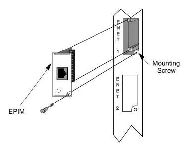
Figure 2-3. Installing an EPIM
